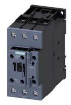
power contactor, AC-3e/AC-3, 80 A, 37 kW / 400 V, 3-pole, 110 V AC, 50 Hz, auxiliary contacts: 1 NO + 1 NC, screw terminal, size: S2  $\,$
