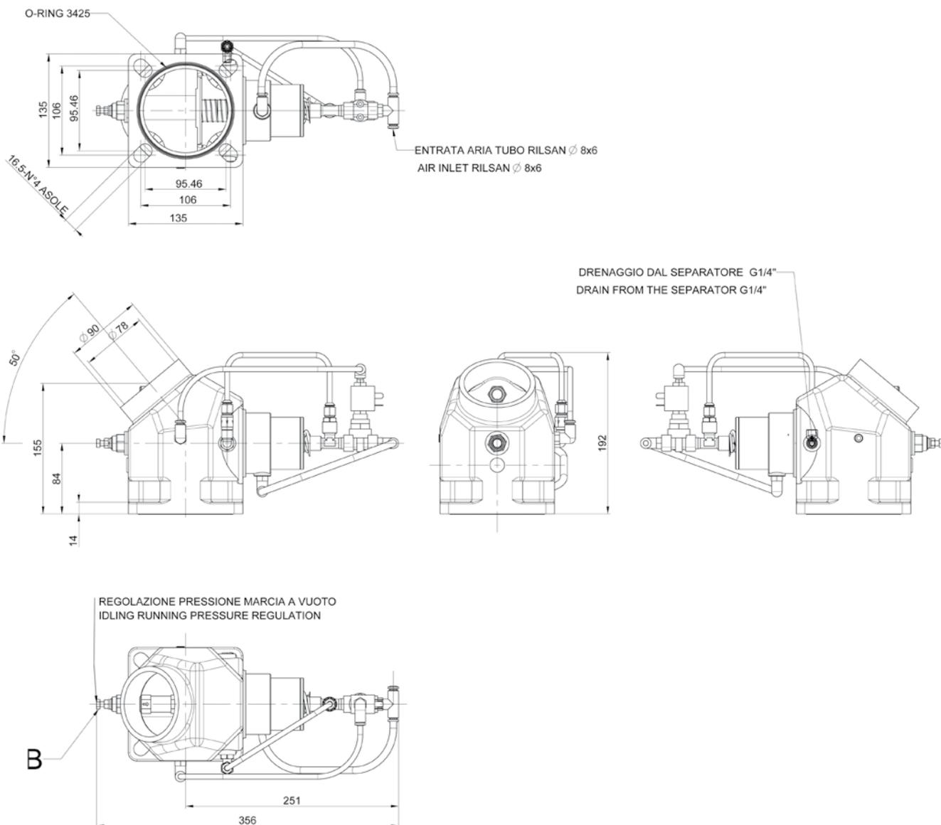
Intake regulator complete with solenoid valve.
