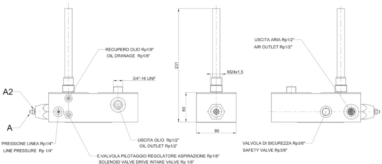
Oil separator block with minimum pressure valve.
